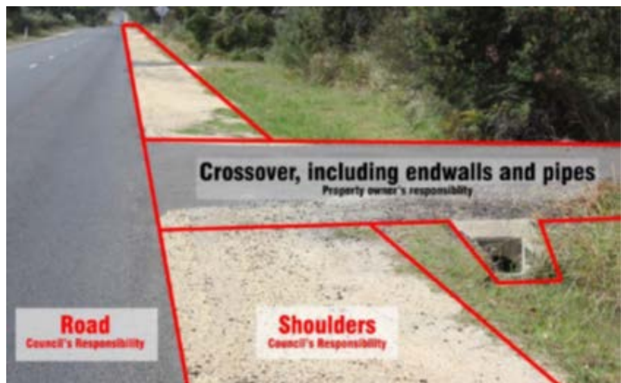
Figure 4 - Typical Vehicle Crossing Layout (Rural)
