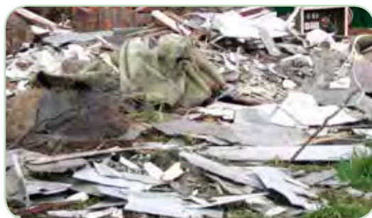
Broken asbestos cement materials from a demolition
