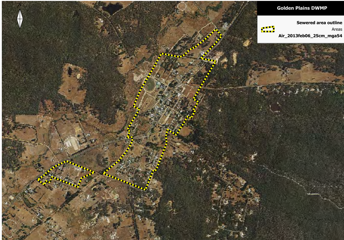
Figure 4-2: Smythesdale seweraged area
