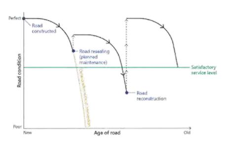
FIGURE 1F: Road deterioration graph
