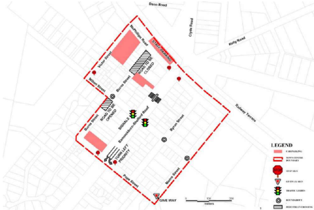
Figure A-4 Recommended intersection treatments
