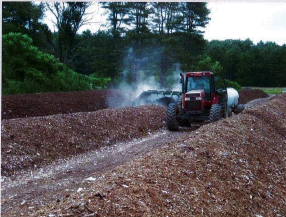
Above: Compost windrows and a small windrow turner in operation. Note the steam (and odour) rising off the pile as it is turned.
