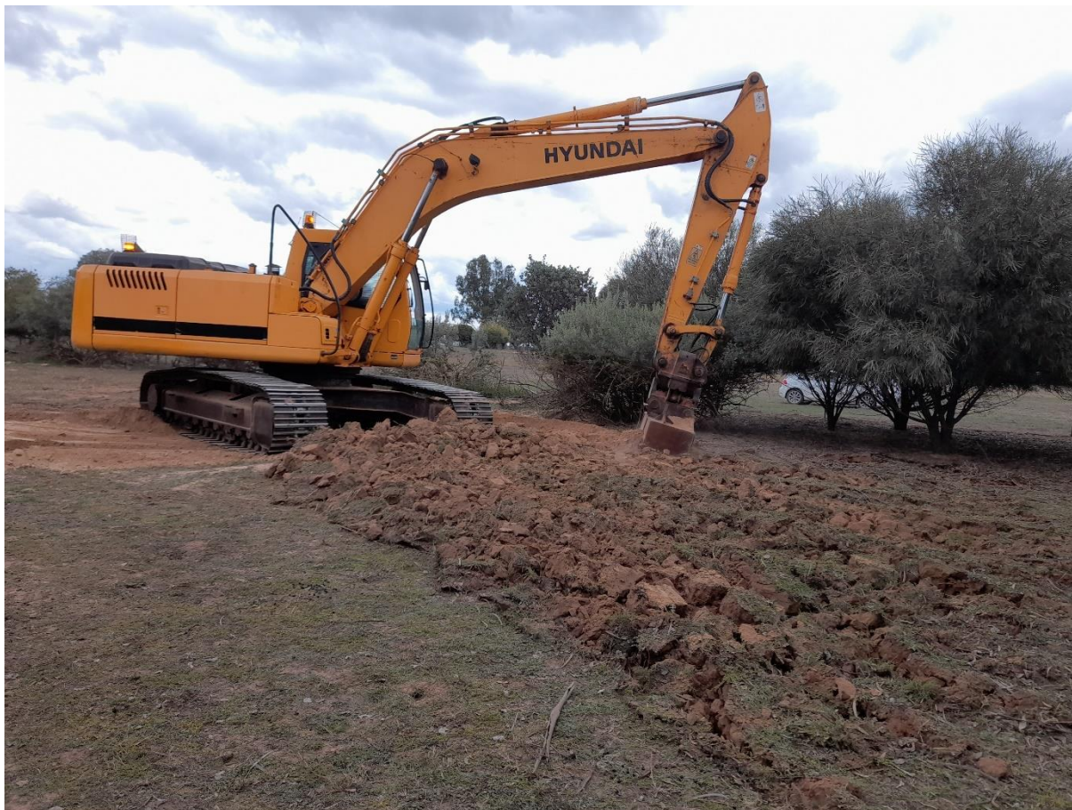
Figure 5: Use of a 20-tonne excavator to rip a long established and deep warren.
