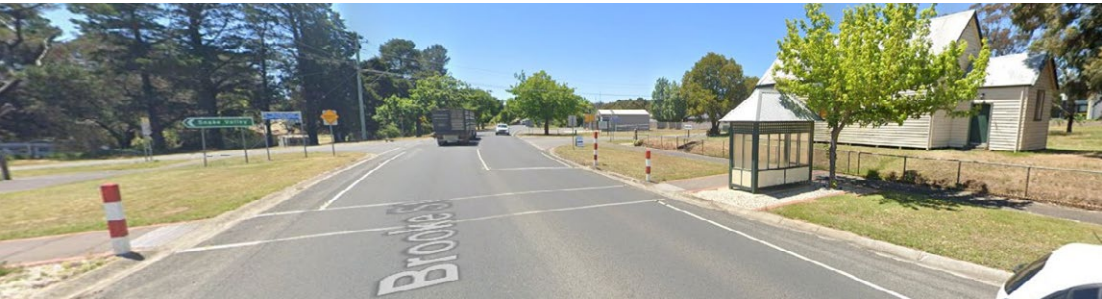
Crossing & seating near church Crossing is poorly defined, zebra/coloured linemarking required. Introduce garden bed and lighting bollards to seating node.
