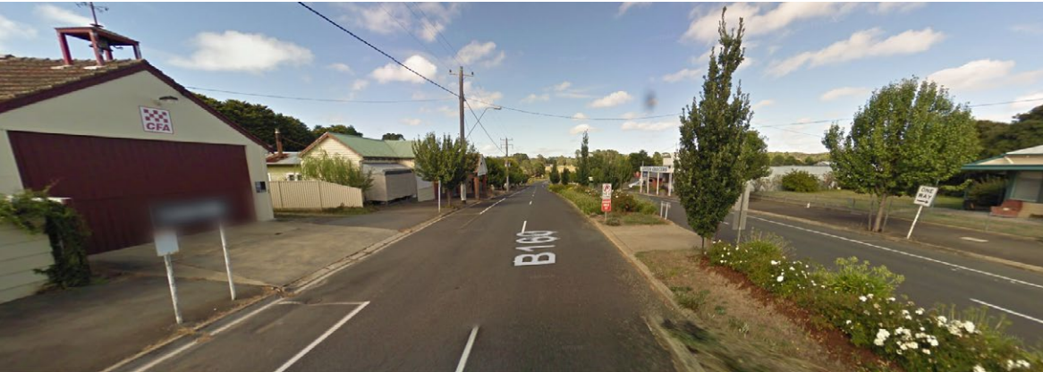
Pedestrian crossing No linemarking to pedestrian crossing. Opportunity to introduce garden bed at crossing and infill planting to median strip
